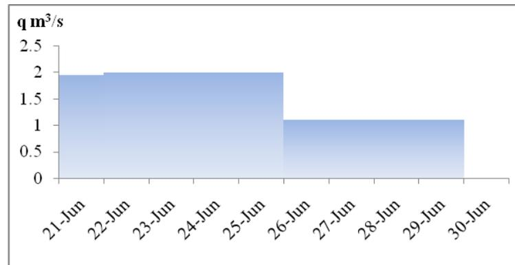
Figure 3. Delivery schedule for the canal with a variable supply
