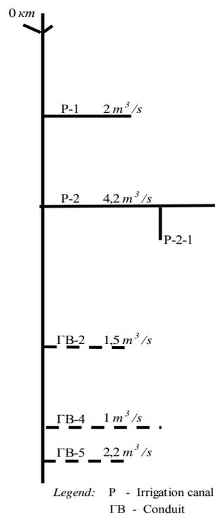
Figure 1. Layout of the main canal of "Stryama-Chirpan" Irrigation system
